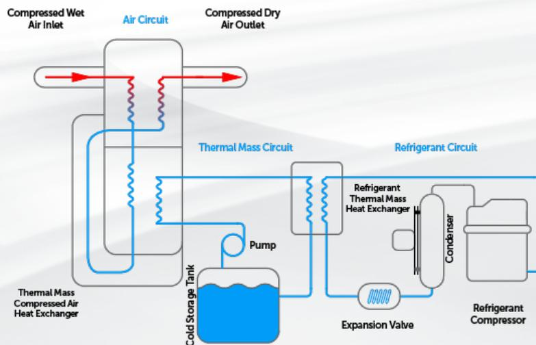
Moisture saturated Compressed Air from the Air Compressor enters a Particulate Pre-Filter then into the Thermal Mass Dryer-Compressed Air Travels through our a Coalescing Pre Filter and then 3 in 1 Heat Exchanger.
